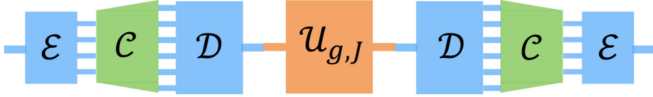
Figure 5. Optimal single-use rotation converter. The figure illustrates the simulation of a single use of a spin- K rotation gate U_{g,K} using a spin- J rotation U_{g,J} for the J \geq K case. A sequence of operations are performed on any input system of U_{g,K} to change its spin: first, the encoding channel \mathcal{E} embeds the spin- K system into a system of 2K spin-1/2 systems (qubits). Then, the universal cloning machine \mathcal{C} optimally turns 2K qubits into 2J qubits. Finally, the decoding channel \mathcal{D} merges 2J qubits into a single spin- J system. The system's spin now fits the spin- J rotation. After applying U_{g,J} , the same sequence of operations is performed in reverse order and input-output spins. A similar sequence of operations allows us to achieve conversions with K > J , the only difference being that one has to replace the universal cloning with a universal discarding, corresponding to the partial trace over 2K - 2J qubits.
